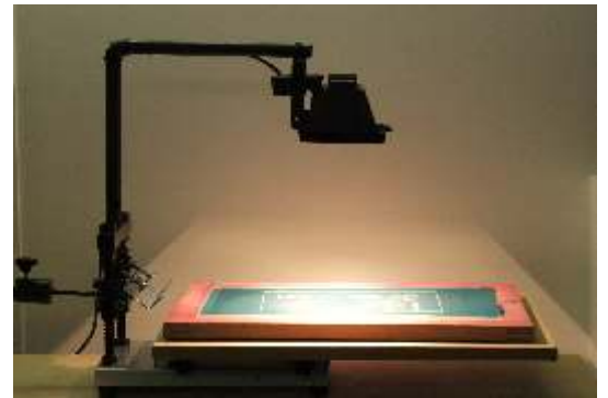
Screen Printer with built-in exposure light for making your own screens.
